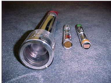
Figure 4.1 Three generations of camera tubes. The largest one is an image orthicon (IO). It was the mainstay of early black-and-white cameras and the first couple of generations of color cameras. The middle tube is a Vidicon. Much simpler in design and more dependable than the IO, it had lower sensitivity and resolution. Thus it was relegated to "industrial" grade cameras — although at least one broadcast color camera used a mix of IOs (for luminance) and Vidicons (R.G.B). The third tube is a Plumbicon, the final generation of broadcast imaging tubes. This tube had a number of derivatives. The Plumbicon had good sensitivity and resolution, and tended not to burn images into its target.
