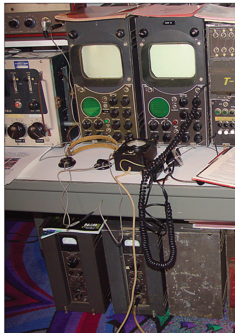
Figure 4.5 Early remote production equipment. On the floor under the table at extreme left and right are the power supplies for two TK-30 cameras (a spare is sitting second from left). The other two cases are a sync generator and its power supply. Sitting on the table from left is an audio mixer, two camera control units, a video switcher and a program monitor. (Source: Chuck Pharis collection on display/NAB2002)
