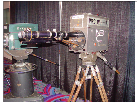
Figure 4.3 Another TK-30 with an early version of a zoom lens. The camera behind this one, a GE PE-11, has an orbiter mounted to its side. (Source: Chuck Pharis collection on display/NAB2002)
